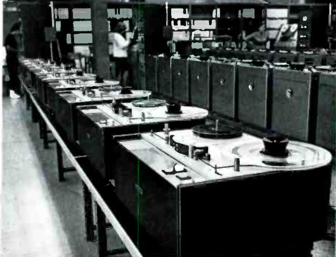
Fig. 2. This line of ten cassette duplicators can produce as many as 10,000 albums a day if it is operated on an around-the-clock basis.
