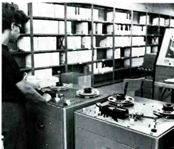
Fig. 1. These two Ampex 3300 mastering units, using 1/2 inch tape, feed a line of ten cassette duplicators. Continuous tape duplicating is possible with the two masters operating alternately. All illustrations have been made at the Ampex facility in Elk Grove Village, Illinois.
